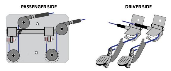
FAST controls can be adapted to various configurations including automatic transmission (single wide pedal) and can be supplied with a dual accelerator made specifically for the UK driver training market.
