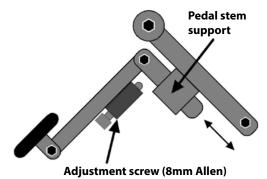
Make sure that pedal stem can be inserted and removed easily from the pedal stem support. If necessary, clean off excess finish and lubricate.
