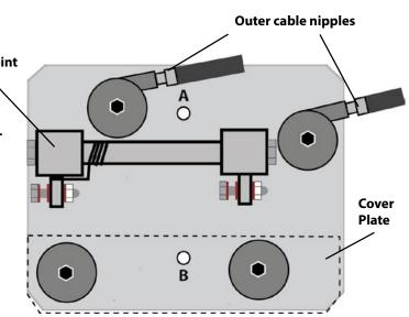
Check outer cable nipples fit into sockets smoothly. Clean off excess powder coat finish if needed. Rebore 10.5mm holes (A & B) if necessary to remove excess finish.
