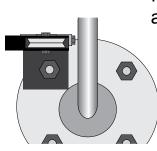
It is often possible to locate the pulley blocks on an existing vehicle bolt (minimum 8mm diameter) or fashion a pulley support that can be attached to a convenient fixing point in the driver footwell.
