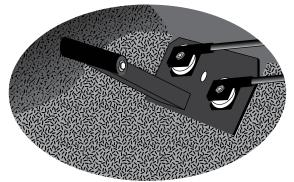
The same effect can be achieved using the X cut in the main carpet, and fitting a car mat around the control unit. Make sure the pedal stem/arm will clear the carpet.
