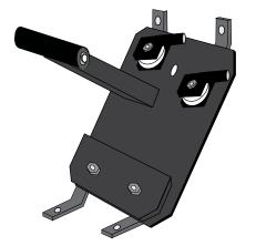
Metal brackets can be welded to the underside of the control unit.
